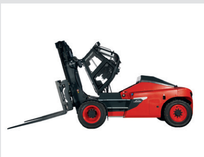
Engine access through tiltable cabin
