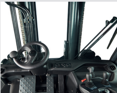
Linde Load Control and steering wheel
